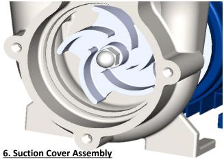
Place the #10 suction cover onto the housing. Using a 7/16" socket, tighten (6-9 ft. lbs.) (5)
