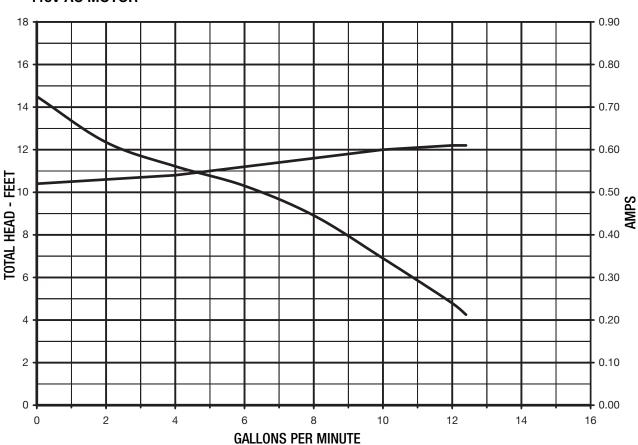
12V DC MOTOR FOR 24 V DC MOTOR DIVIDE AMPS BY TWO
