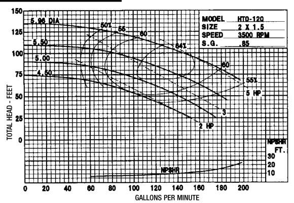
Horsepower requirements based upon 0.85 specific gravity. Calculations can be applied for fluids of other specific gravities.
