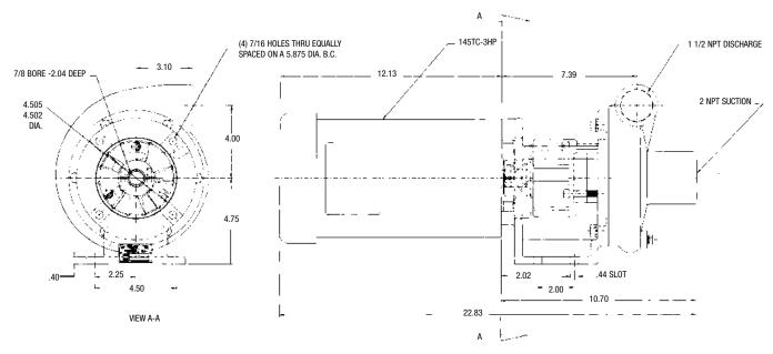
Pump dimensions certifiable for construction purposes. Motor dimensions dependent upon motor manufacturer.
