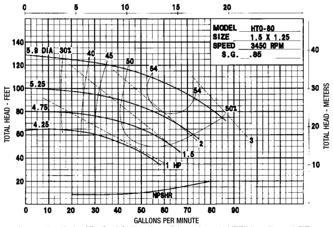
Horsepower requirements based upon 0.85 specific gravity. Calculations can be applied for fluids of other specific gravities.
